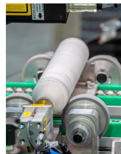
Autosonic™ mini+ Auto: laser 3D system for engraved cylinder data recognition.
