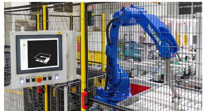
Autosonic™ mini+ Auto: loading/unloading system.
