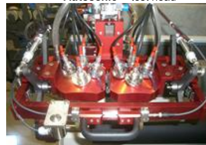
Autosonic ™ double test head
